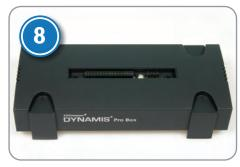
8:The Pro Box is a module built with the same casing as the command station. There are two multi pin connectors in the top. The 8-pin connector on the right is used to set the BaseID address if the system is used within range of another Dynamis system.
