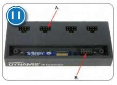
II: Key to expanding the IR Receiver network is the IR Extension module that sits atop the command station. It allows up to five IR Receivers to be connected to the system including one located directly on top of the command station.
