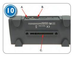
10:A view of the underside of the command station. It sits on the Pro Box when one is used and communication between the two is by a multi-pin connector in the base of the command station (C). Note the power supply port (A) and track power bus port (B).
