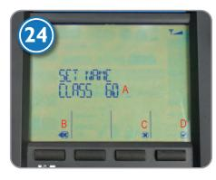
24: Renaming a locomotive for simple identification in the roster stack.
