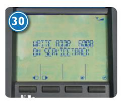
30:A second setting offers programming or service track programming of the locomotive address.
