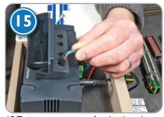
15:To improve coverage for the throttles, an additional receiver was installed using an IR Extension box and cable.
