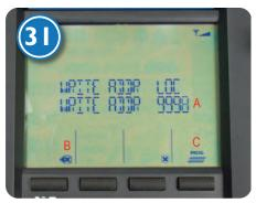
31: Selecting a new address, using figures 0-9999 via service track programming.
