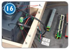
16:The setting up is complete with IR Extension box and cable (A) plugged into the Command Station that sits on top of the Pro Box. The programming track is plugged into the Command Station (B) and the layout power bus into the track port in the Pro Box (C). The power supply for Dynamis is still plugged into the Command Station box (D).
