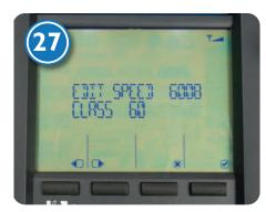
27: Speed step changes are made through the menu – select the edit speed screen. Changes are specific to the selected locomotive.
