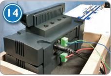
14: Should friends turn up wanting to enjoy the layout, a Pro Box is added enabling the control of up to four trains simultaneously using wireless throttles.
