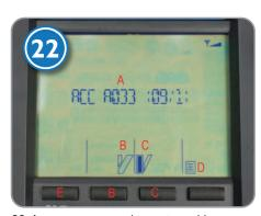
22:Accessory control is activated by pressing the left hand button (E).
