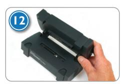
12:The Command Station sits neatly on top of the Pro Box. There are no cable connections between the two and take care not to bend any pins!
