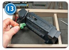
13: Setting up the entry-level package on the Author's N gauge layout Dudley Heath. A small screwdriver is required to connect wires to the screw connectors supplied with Dynamis.
