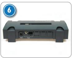
6:The Command Station unit supplied with the entry point set is the heart of the system even when a Pro Box is attached. The ports in the rear are simple: a power supply and two outputs for track power bus offering two options for making a connection to the layout. Note that there is no separate programming track port – the track output port becomes the programming (service) track port when a Pro Box is added.
