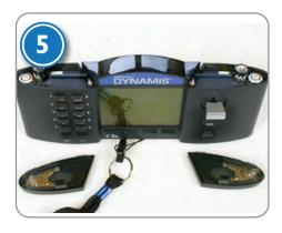
5:You will need batteries for the handset! While the first set of batteries are supplied with the handset, rechargeable batteries will be the best solution in the long term. Should there be a need to store the system for any period of time, remove the batteries to save power and reduce the risk of leakage.
