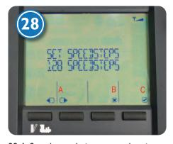
28: A: Speed step choices are made using the selection buttons.
