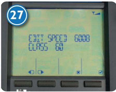
27: Speed step changes are made through the menu – select the edit speed screen. Changes are specific to the selected locomotive.
