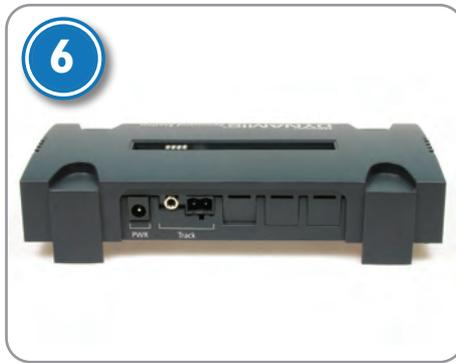
6: The Command Station unit supplied with the entry point set is the heart of the system even when a Pro Box is attached. The ports in the rear are simple: a power supply and two outputs for track power bus offering two options for making a connection to the layout. Note that there is no separate programming track port – the track output port becomes the programming (service) track port when a Pro Box is added.
