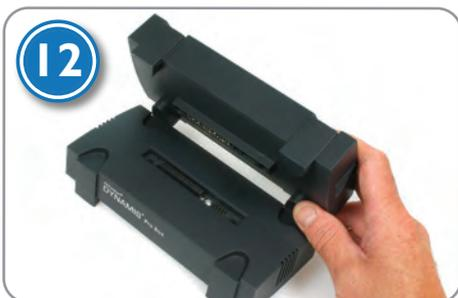
12: The Command Station sits neatly on top of the Pro Box. There are no cable connections between the two and take care not to bend any pins!
