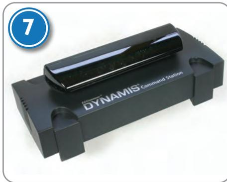
7: The IR receiver sits on top of the command station when set up in entry-level mode.
