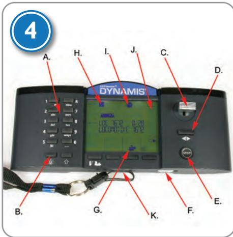
4: The same handset (throttle) supplied with the entry level set is used when the system is upgraded with Pro Box. Features of the wireless IR handset include:
