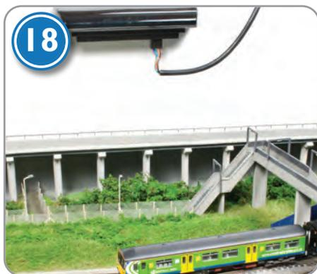
18: The additional IR Receiver is located for maximum coverage. It is important to have clear lines of sight between the receivers and handsets to minimise the risk of signal loss.
