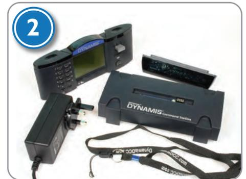
2: The Bachmann Dynamis entry-level system is a 2.5 amp set which includes a command station, receiver, hand held wireless throttle and wall mount power supply. This article looks at the fundamentals of Dynamis and how to put it to work.
