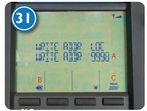
31: Selecting a new address, using figures 0-9999 via service track programming.
