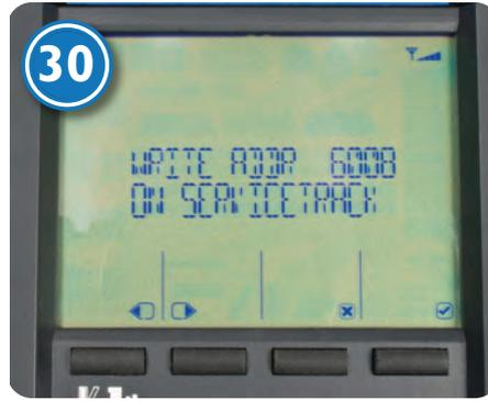
30:A second setting offers programming or service track programming of the locomotive address.
