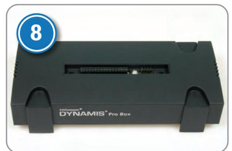
8: The Pro Box is a module built with the same casing as the command station. There are two multi pin connectors in the top. The 8-pin connector on the right is used to set the BaselD address if the system is used within range of another Dynamis system.
