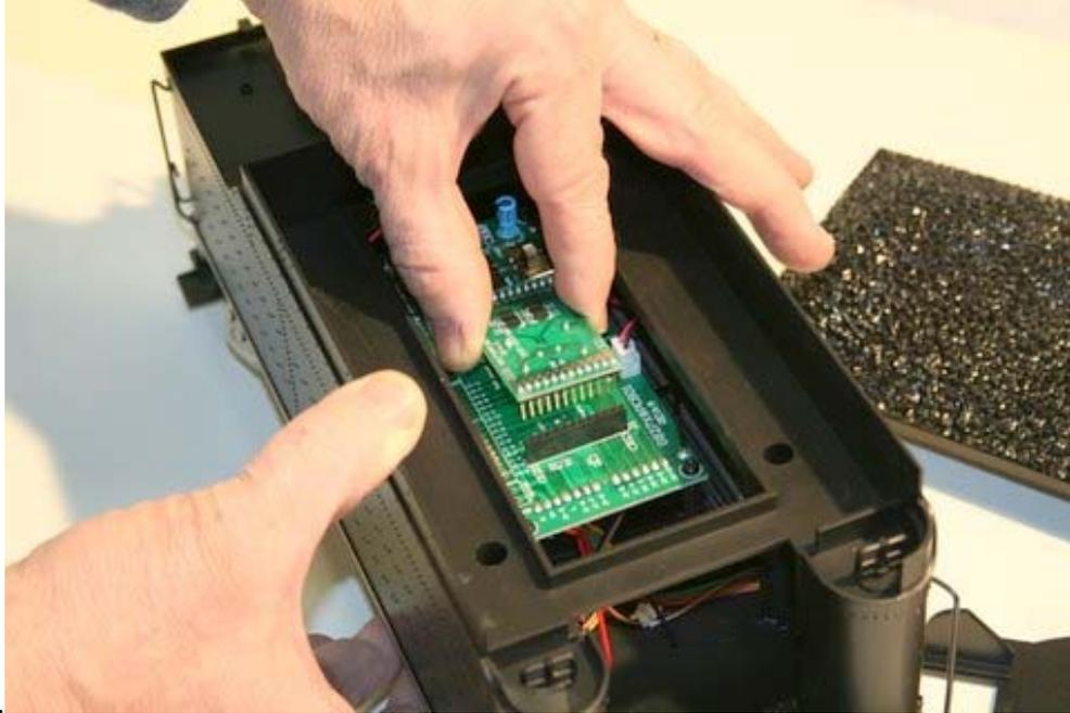
Once removed from the tender, the (DC) Dummy PC Board needs to be prepared for use with the 2K2.
