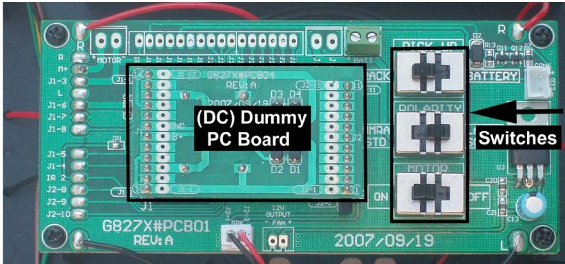
The following installation instructions are provided to gain the full benefits of the socket in the K27 when used with the Phoenix 2K2 DC sound board. The Phoenix 2K2 sound board can be used with DC, DCC, and RC installs. This example set of instructions is for a DC install.
