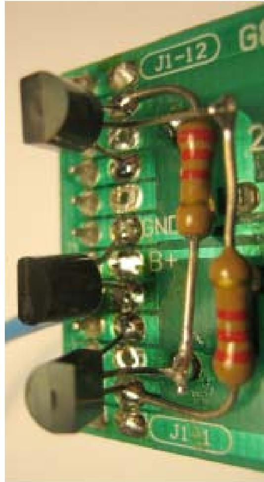
1. Install three 2N2222 or equivalent NPN transistors as shown in the circuit diagram and photo above
